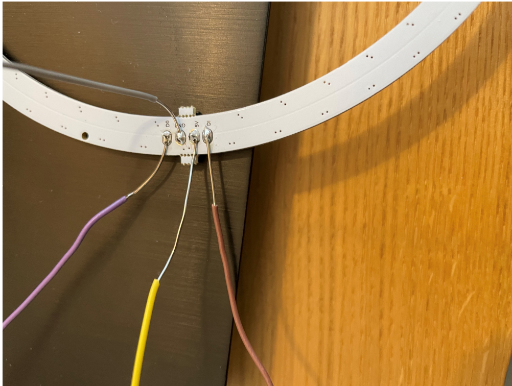
Figure 17: Soldered pins of the led ring
